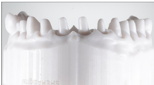
Fig, 16, 3 D printed Alveolar model
